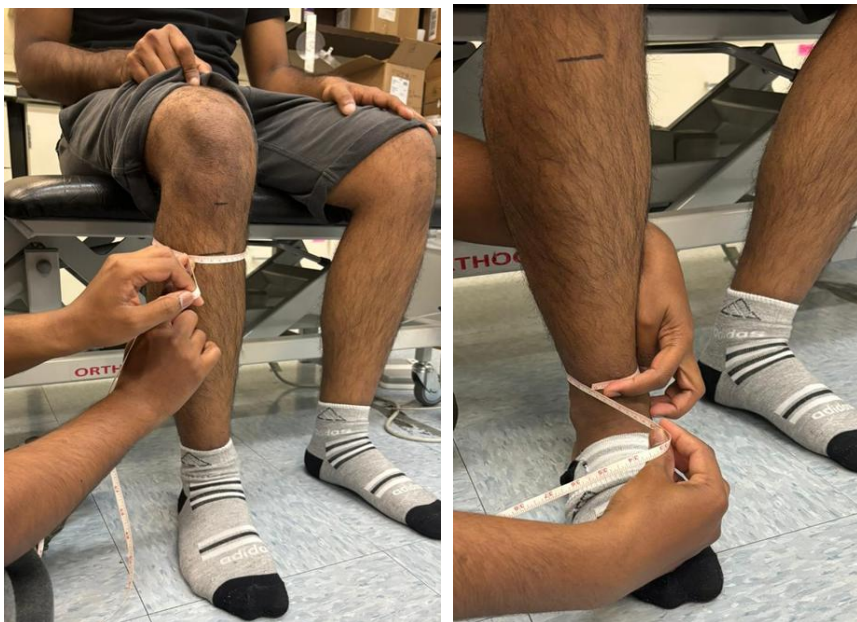
Figure 4: Measurement setup for calf (left figure) and ankle (right figure) circumferences.
