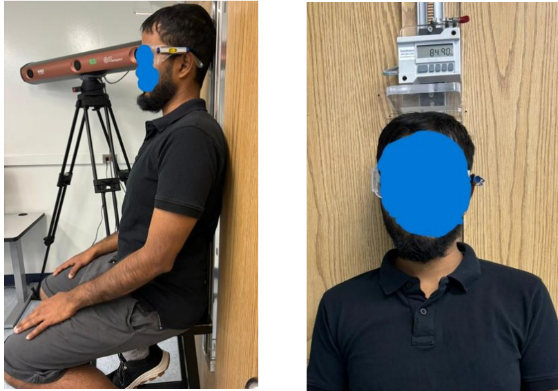
Figure 3: Standardized seated posture for spine height measurement by stadiometer, with head alignment maintained using bubble-inclinometer goggles (left: from side view; right: from front view).
