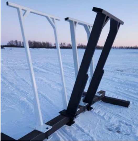
Figure 4. ROPS Designs (left to right): 2 x 2, 2 X 6, 2 X 4.
